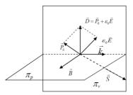
Fig.I.2. The orientation of the vibration surface and of the polarization surface in an anistropic media
