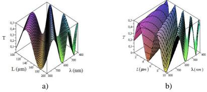
Fig.III.4. Transmission factor vs L vs $\lambda$  for a)quartz b)calcite
