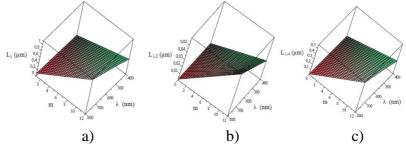
Fig.III.1. The thickness of the quartz layer (a), calcite(b+c) as a plate: a) $\lambda$ ; b)  $\lambda/2$  and c) $\lambda/4$  based on  $\lambda$  and on the interference order *m*
