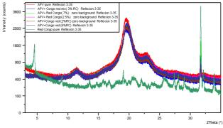
Fig.II.8. Crossed diffractograms of pure PVA samples, of the pure CR and PVA+RC with various concentrations.
