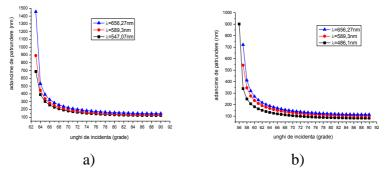
Fig.III.3.The variation of an evanescent wave with the incidence angle for different wavelength at the crossed surface a) quartz-living cell; b) calcite-living cell
