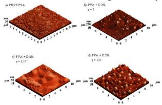
Fig.II.12. AFM images for a) pure PVA; b) PVA+D2% for extended foils ( $\gamma = 1$ ); c) PVA+D2% ( $\gamma = 1,17$ ); d) PVA+D2% ( $\gamma = 1,4$ )
