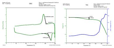
Fig.IV.5.The PVA thermogram
