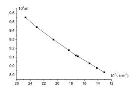
Fig.II.4.The variation of quartz's birefringence with the wave's number
